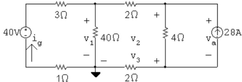
$$\frac{v_1}{40} + \frac{v_1 - 40}{4} + \frac{v_1 - v_2}{2} = 0 \quad \text{so} \quad 31v_1 - 20v_2 + 0v_3 = 400$$
