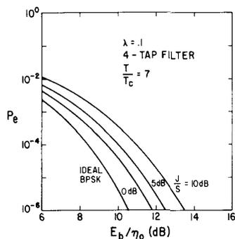
Fig. 19.  $P_e$  versus  $E_b/\eta_0$  for interference centered about carrier frequency.
