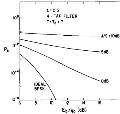
Fig. 20.  $P_e$  versus  $E_b/\eta_0$  for interference centered about carrier frequency.
