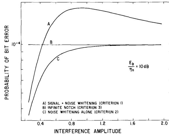
Fig. 8. Tone jammer performance with varying amplitude.
